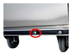
Reinforce both bumpers with carriage bolts so they won't get ripped out easily
