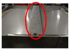
Anchor drop down latch to a reinforced center beam so it won't easily pry off/out of shape
