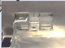
Optional locking mechanism for use with padlocks
